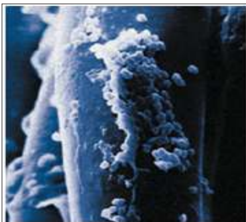
Untreated Polymer shows growth of bacteria on polymer surface
